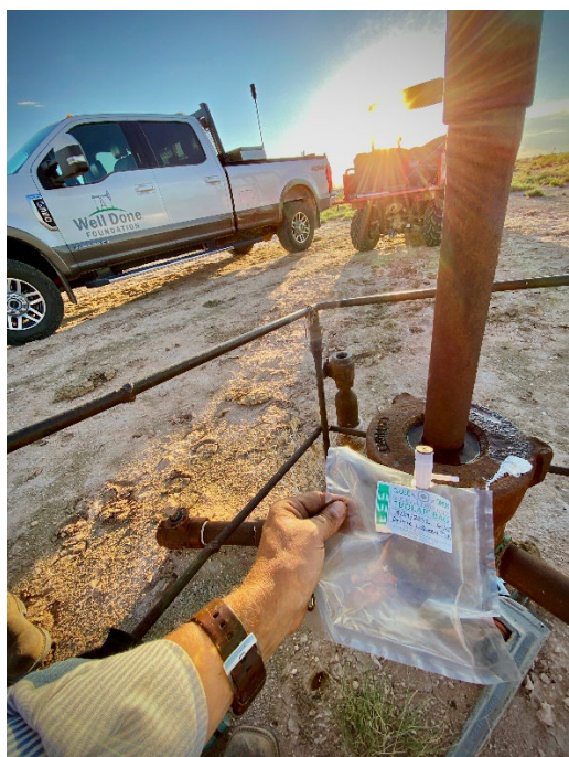
3) DLQ #01K (30-005-60078) – Wellhead & Gas Sample
