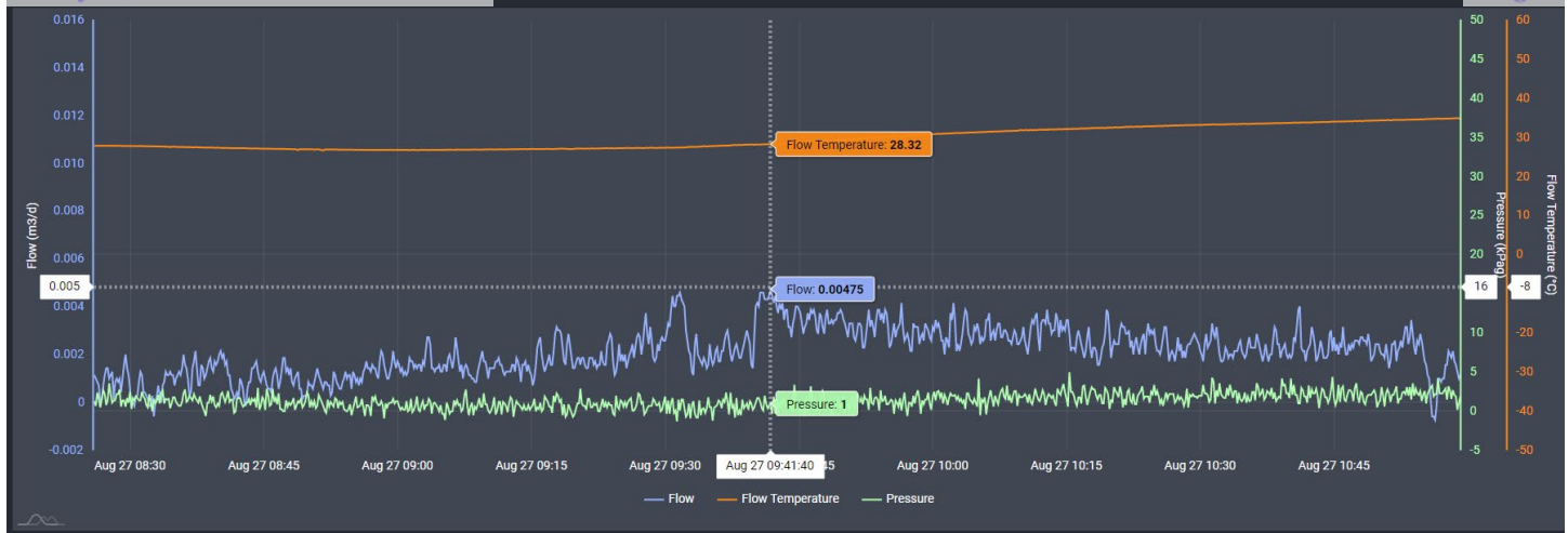
Image 4.1 – Twin Lakes SAU #113 (30-005-616)4) Methane Flow/Pressure/Temperature Timeseries & Peak Flow
