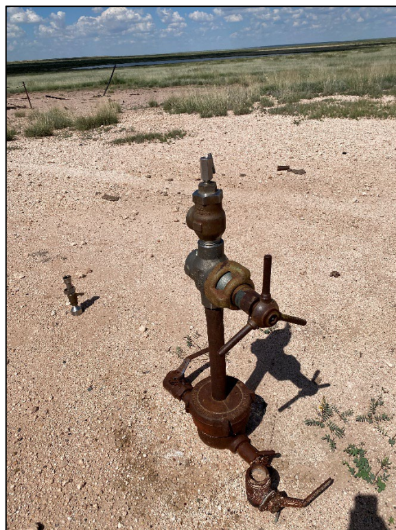
2) Twin Lakes SA #113 (30-005-61604) – Wellhead
