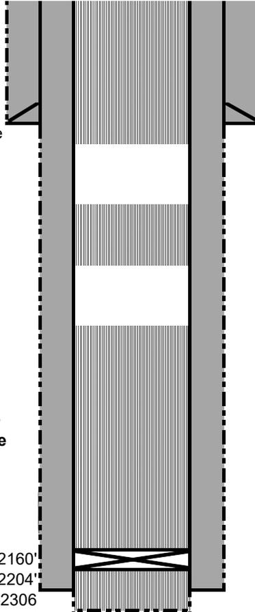
**Plug 4 (Surface casing shoe and surface): Spot balanced plug from 318' to surface.**
