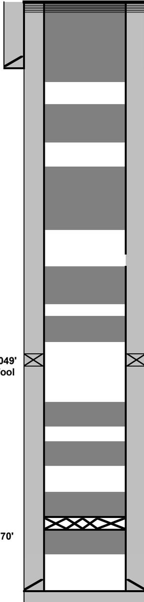
10-11-2022: Cut off WH, TOC; 8' in 5 1/2" casing and 10' in annulus. Install P&A marker. Top off with 18 sx.
