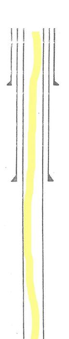
12-1/4" hole 8" PVC pipe set at 200' Cemented with 70 sacks, circulated
