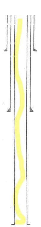
12-1/4" hole 8" PVC pipe set at 160' Cemented with 70 sacks, circulated
