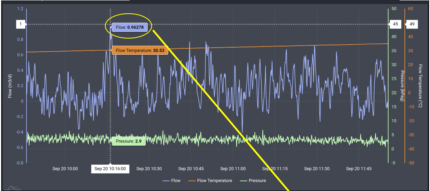
Image 4.1 – Harrison #002 (30-025-24749) Methane Flow/Pressure/Temperature Timeseries & Peak Flow at Interval #1 testing period of 2.2-hours.
