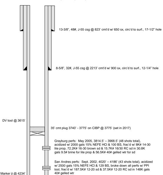
5-1/2", 17#, J-55 csg @ 5039' cmt'd w/ 1075 sx in 2 stages, DV tool at 3615', circ'd cmt on both stages, 7-7/8" hole
