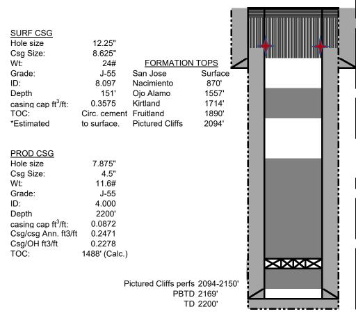
9-1-2022: Cut off WH, TOC at surface. Install P&A marker. Top off with 16 sx.
