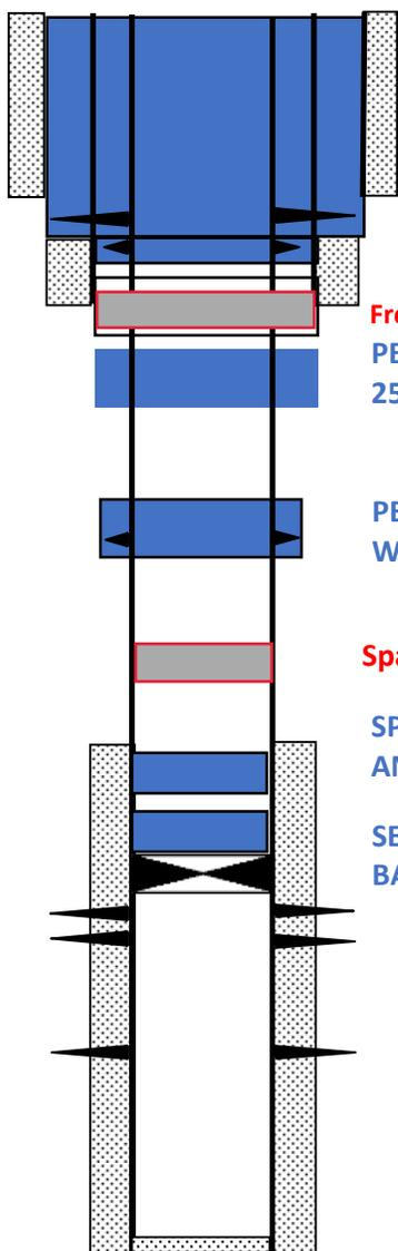
**PERF AT 530' WITH DEEP PENETRATION GUNS. EST CIRC UP INT AND PROD ANNULI. PUMP 400 SX CMT. VERIFY CMT TO SURF. Ensure cement to surface in both annuli**
