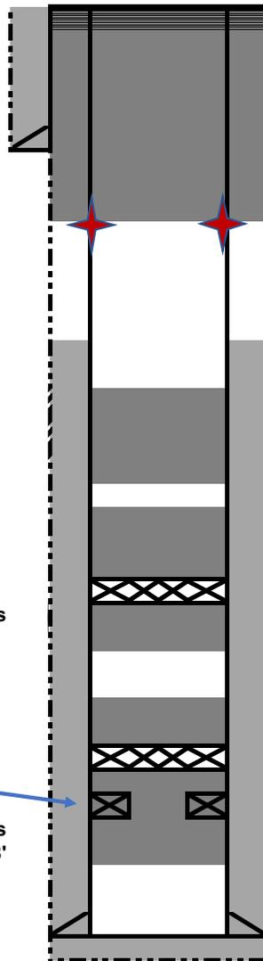
8-15-2022: Cut off WH, TOC at 9'. Install P&A marker, top off casing and cellar with 18 sx.
