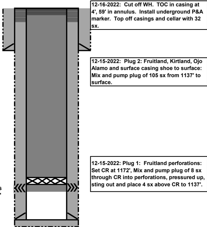
12-16-2022: Cut off WH. TOC in casing at 4', 59' in annulus. Install underground P&A marker. Top off casings and cellar with 32 sx.
