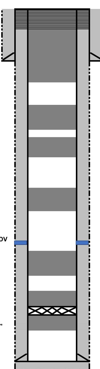
12-1-2022: Cut off WH. TOC 80' in annulus, at surface in casing. Install P&A marker, top off casings and cellar with 70 sx.
