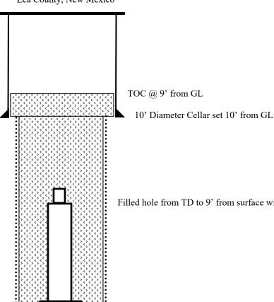
Filled hole from TD to 9' from surface with 14 yd3 (378 ft3) of 20 ppg concrete
