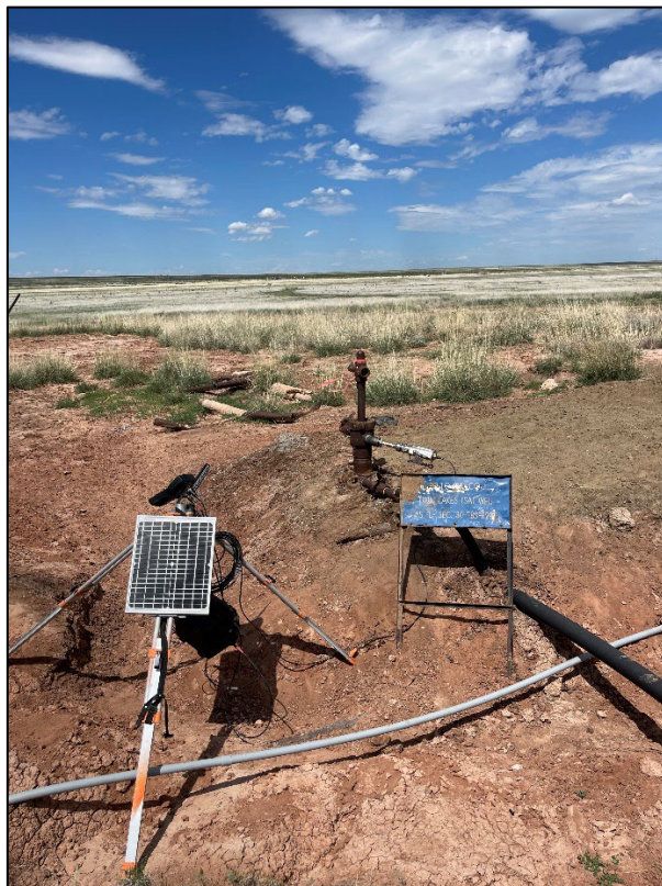
3) TLSA #005 (30-005-60572) - Methane Flow Test Rig Up
