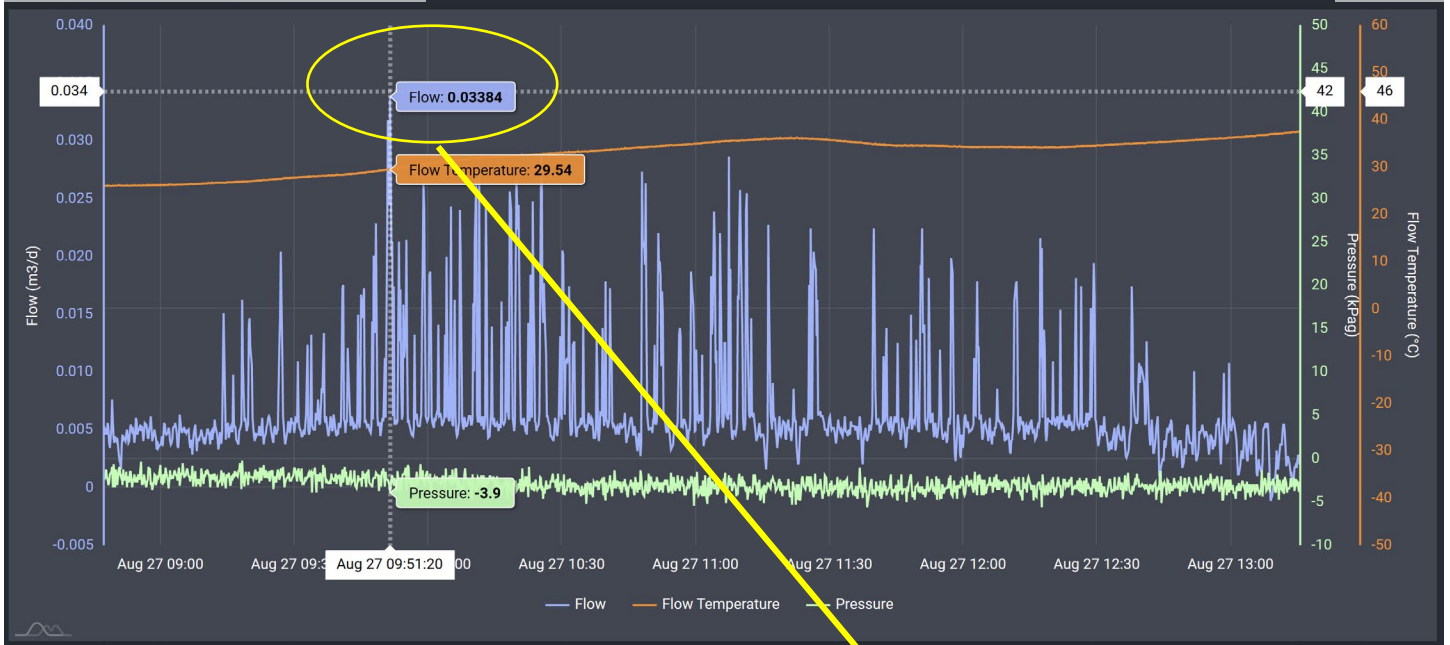
Image 4.1 – TLSA #005 (30-005-60572) Methane Flow/Pressure/Temperature Timeseries & Peak Flow at Interval #1 testing period of 4.5-hours.
