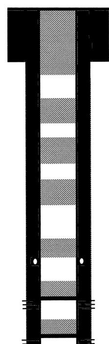
8-5/8" J-55 24# casing @ 212'. Cemented with 135 sks Class B. Circulated cement to surface. Hole size: 12-1/4
