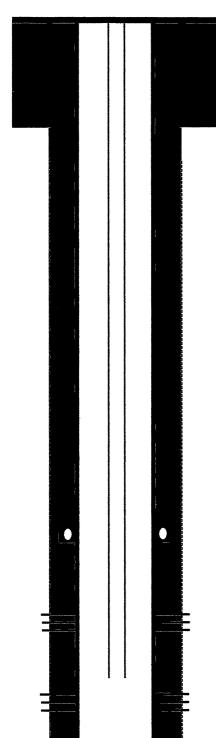
$8\mbox{-}5/8"$  J-55 24# casing @ 212'. Cemented with 135 sks Class B. Circulated cement to surface.
