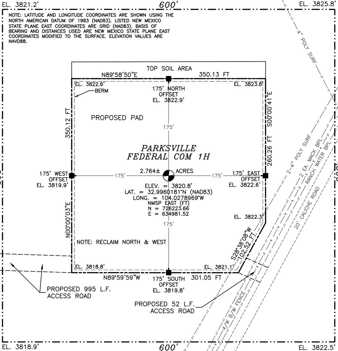
NOTE: LATITUDE AND LONGITUDE COORDINATES ARE SHOWN USING THE NORTH AMERICAN DATUM OF 1983 (NAD83). LISTED NEW MEXICO STATE PLANE EAST COORDINATES ARE GRID (NAD83). BASIS OF BEARING AND DISTANCES USED ARE NEW MEXICO STATE PLANE EAST COORDINATES MODIFIED TO THE SURFACE. ELEVATION VALUES ARE NAVD88.
