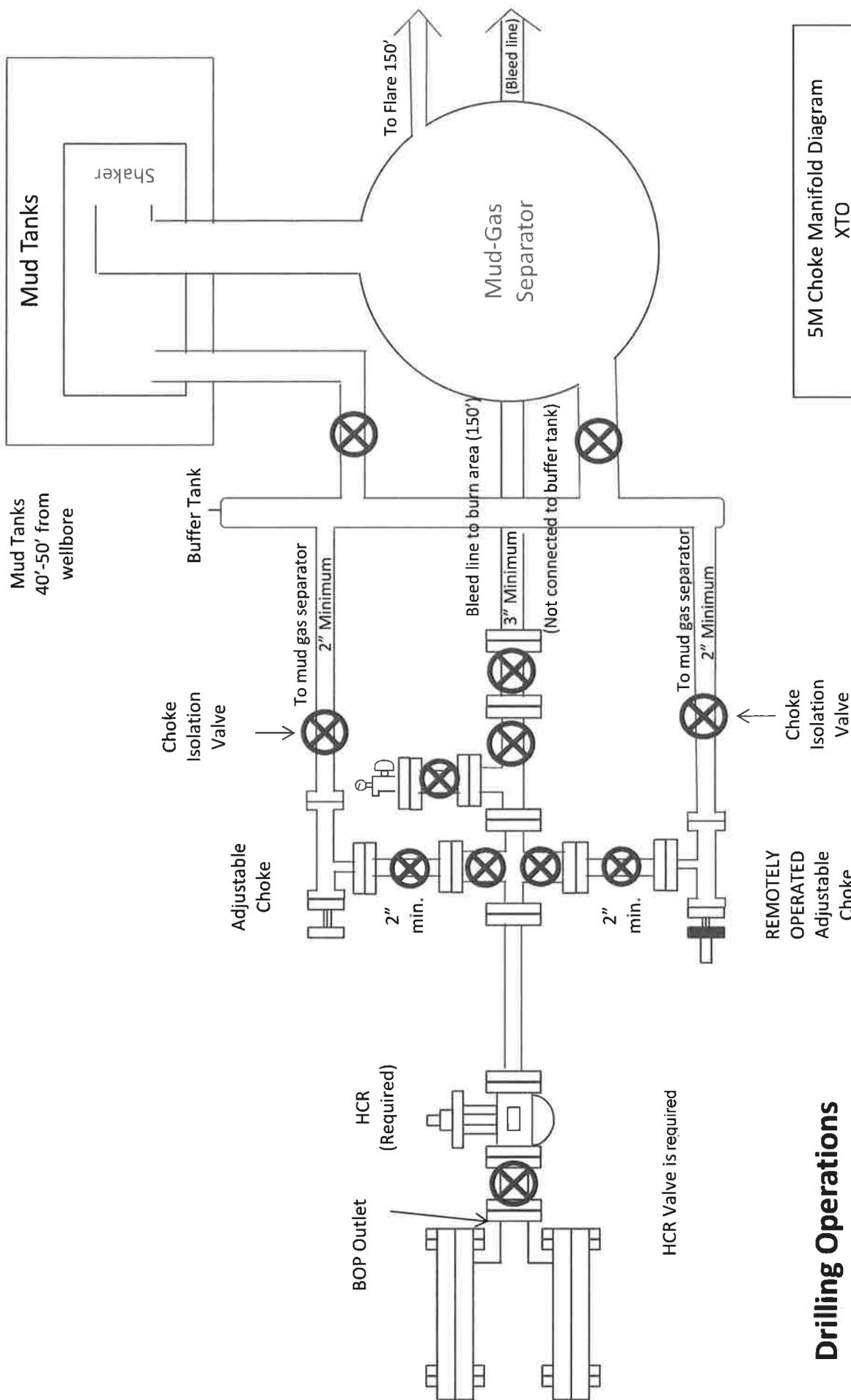
5M Choke Manifold Diagram XTO
