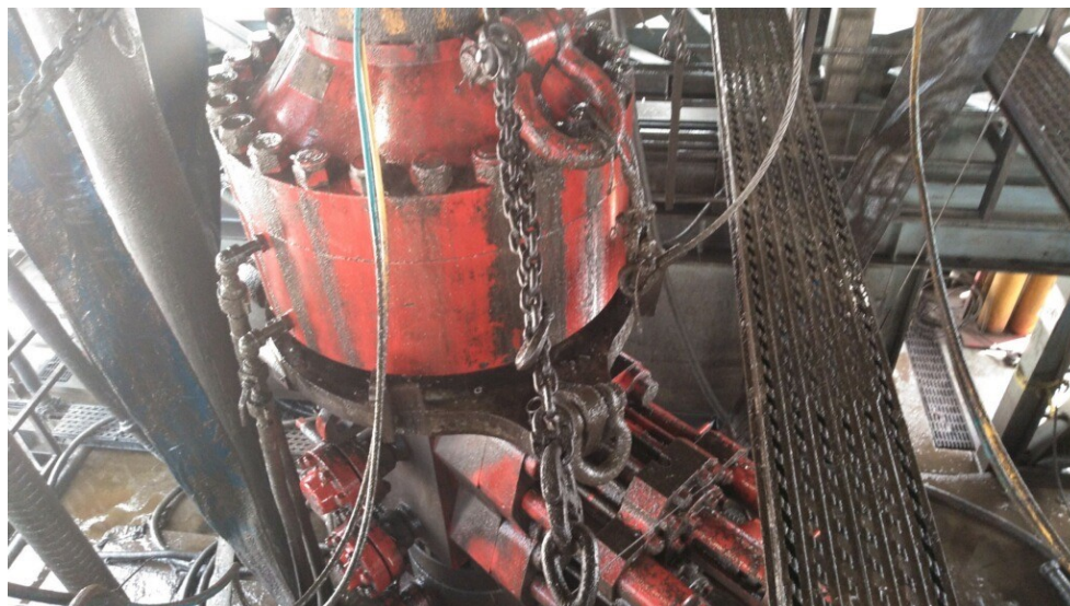
Figure 1: Winch System attached to BOP Stack
