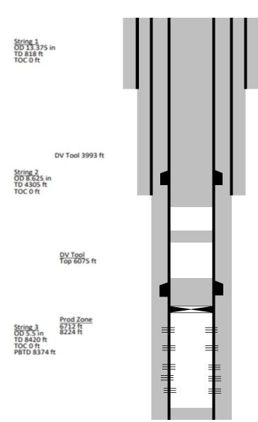
PUMPED 235SX CL C TO SURFACE. VERIFIED.
