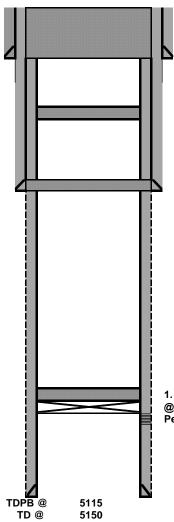
13 3/8 48# CSG @ 322 4. Perf'd @ 372'. Pressured up on perf to 500 PSI. Spotted 55 sx class C cmt @ 422' to surface.
