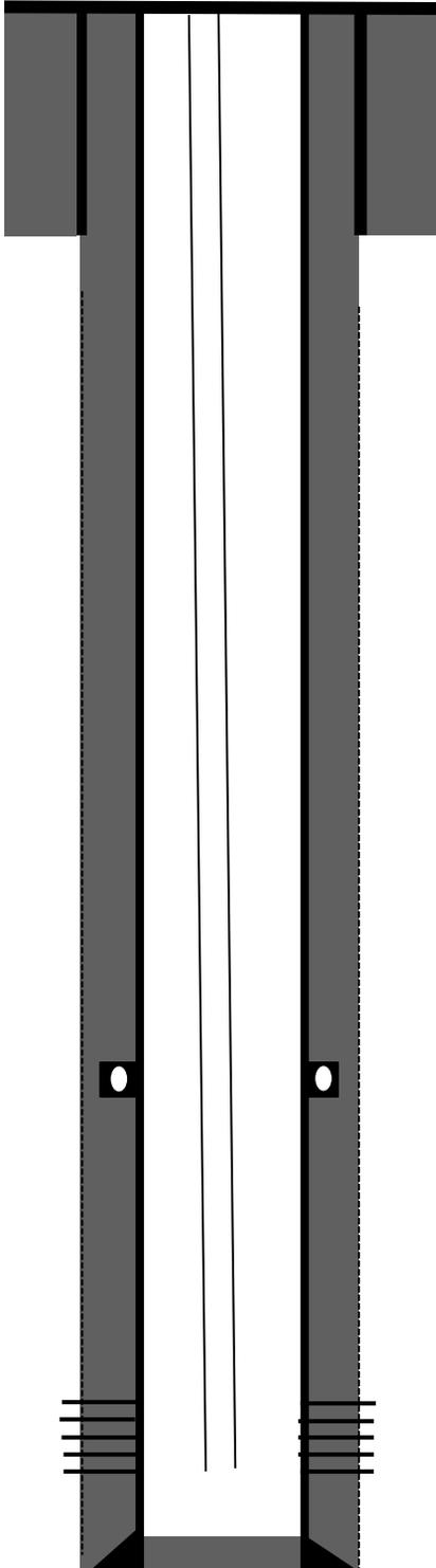
8-5/8" 24# casing @ 217'. Cemented with 150 sks, Class B cement w/ 2% CaCl<sub>2</sub> (172.5 Cu.ft). Circulated cement to surface. Hole size: 12-1/4"
