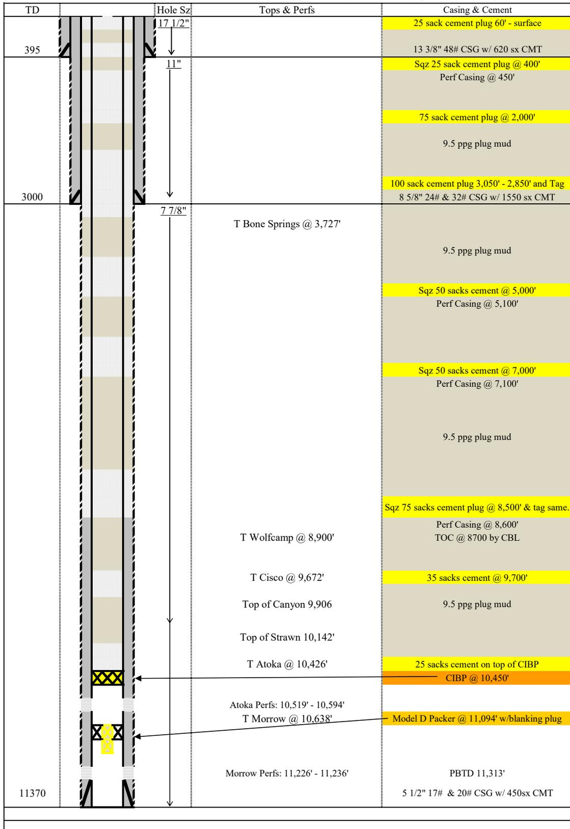
REMARKS: Wellbore after Plugging and abandonment Operations. 9.5 ppg mud laden fluid will be placed between plugs.
