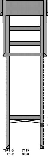
5. Perf'd @ 430'. Established injection rate @ 1 BPM @ 300 PSI w/ 25 bbls H20, no circulation to surface. Perf'd @ 200'. Established injection rate @ 1 BPM @ 300 PSI w/ 7 bbls H20, no circulation to surface. Spotted 50 sx class C cmt @ 480' to surface. Gravity sqz into 8 5/8 annulus.
