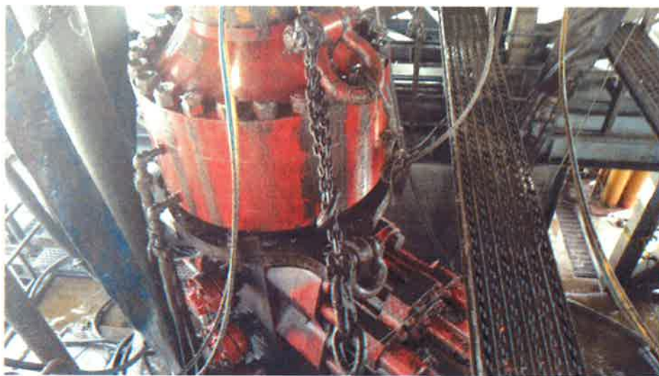
Figure 1: Winch System attached to BOP Stack
