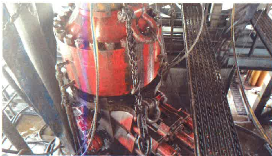
Figure 1: Winch System attached to BOP Stack
