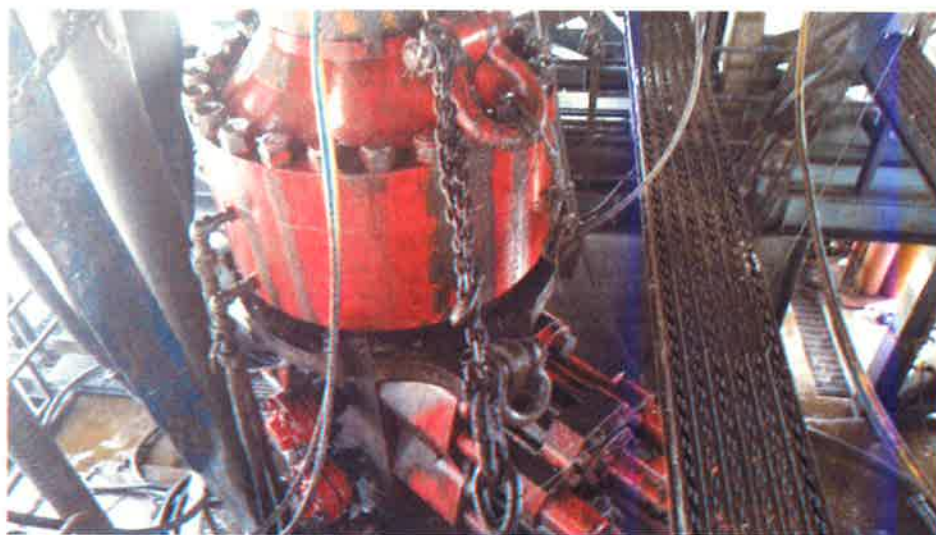
Figure 1: Winch System attached to BOP Stack
