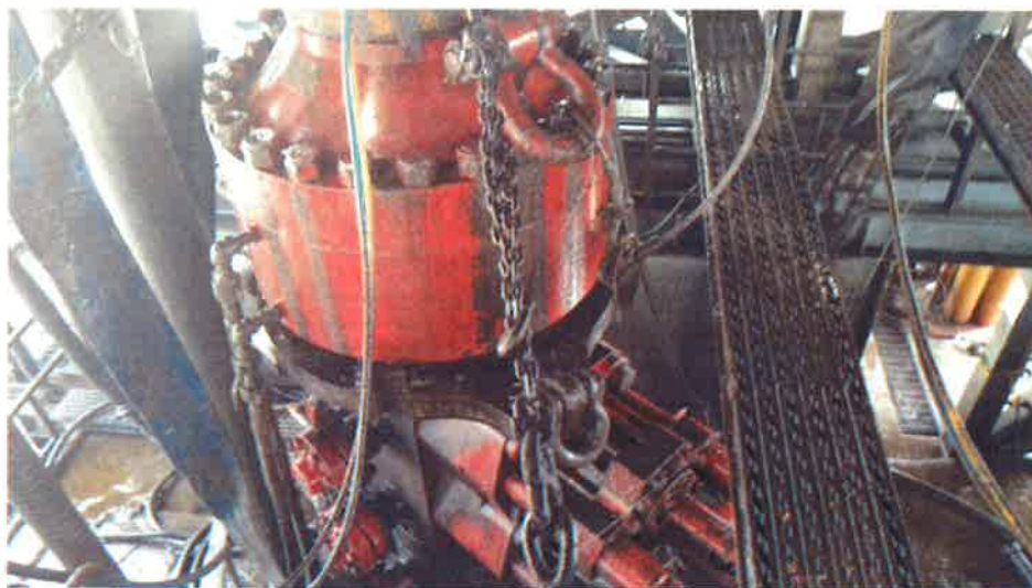
Figure 1: Winch System attached to BOP Stack
