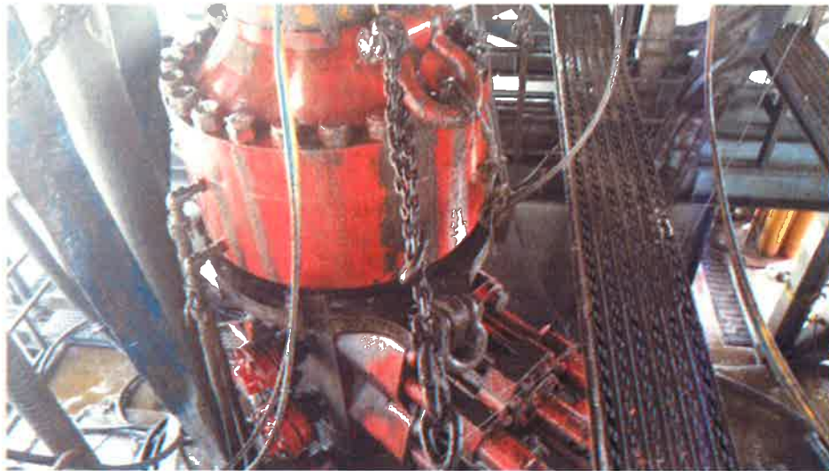
Figure 1: Winch System attached to BOP Stack
