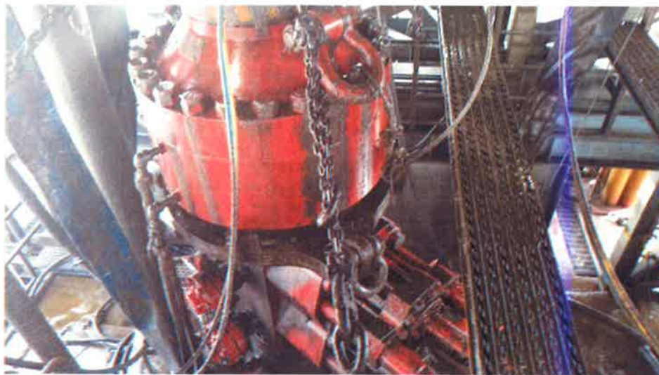
Figure 1: Winch System attached to BOP Stack
