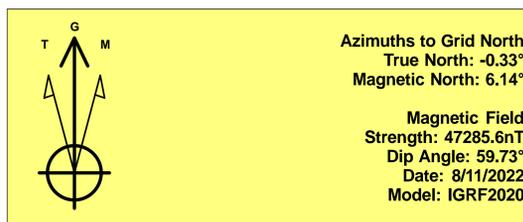
To convert a Magnetic Direction to a Grid Direction, Add 6.14°
