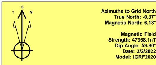
To convert a Magnetic Direction to a Grid Direction, Add 6.13°
