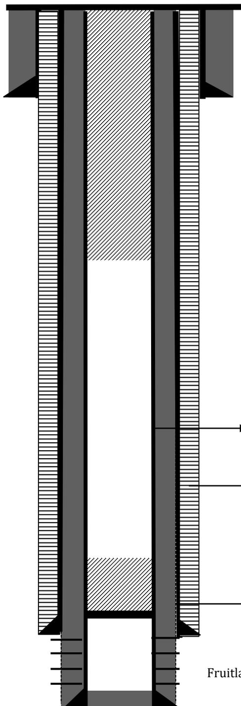
13-3/8" 48# H-40 casing @ 128'. Cemented with 175 sks Class G cement w/ 3% CaCl2 . Total 201 Cu.ft. Circulate 35 cu.ft to surface. Hole size: 17 1/2".
