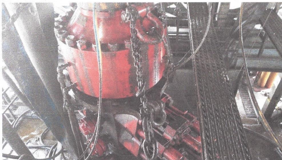
Figure 1: Winch System attached to BOP Stack
