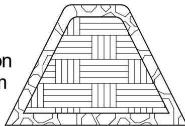
Properly constructed foundation consisting of a level base free of rocks, debris, sharp edges or irregularities to prevent punctures cracks or indentations to the tank bottom.
