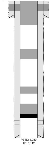
2/24/23: Perf @ 291', est injection Spot 53 sx Class C f/ 530' - 0' Squeeze additional 50 sx thru perfs
