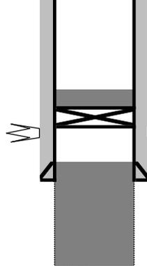
**2950'. Leak test CIBP 500psi, 30mins**
