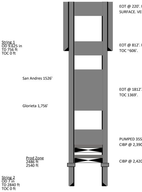
EOT @ 220'. PUMPED 40SX CL C TO SURFACE. VERIFIED.
