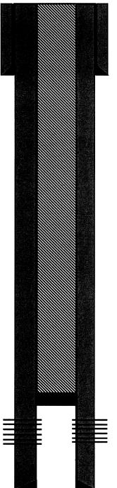
5 ½", 15.5# Casing Set @ 107'. Cemented w/ 35 sks Cement. Circulate cement to surface. Hole size 8-3/4"
