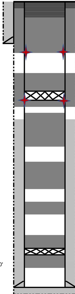
2-1-2023: Cut off WH. TOC, 25' in 5 1/2" casing and 8' in annulus. Install P&A marker, top off cellar and casings with 28 sx.
