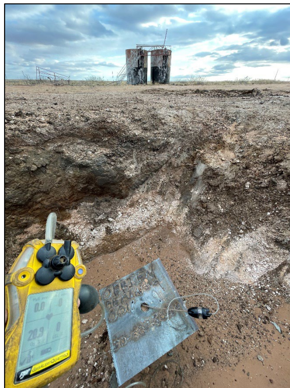
2) O'Brien Deming 6 #001 – Post Plugging Field Gas Analysis
