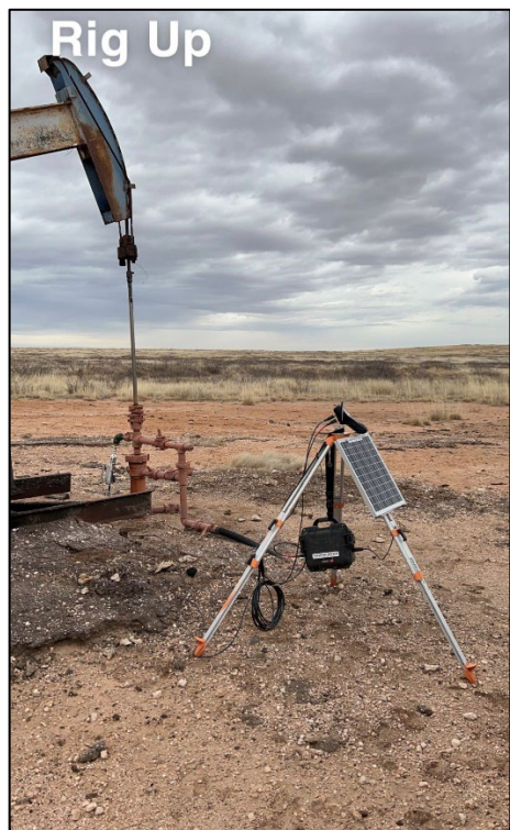
1) O'Brien Fee 18 #004 – Pre Plug Methane Measurement
