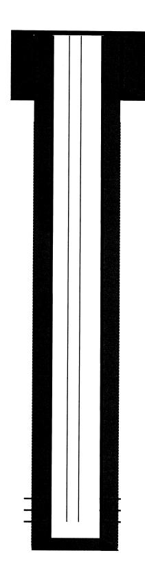
8-5/8" 24# casing @ 137'. Cemented with 100 sks Class B cement w/2% CaCl2 . Hole size: 12 1/4". Circulate cement to surface.
