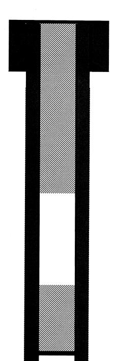
8-5/8" 24# casing @ 137'. Cemented with 100 sks Class B cement w/2% CaCl2 . Hole size: 12 1/4". Circulate cement to surface.
