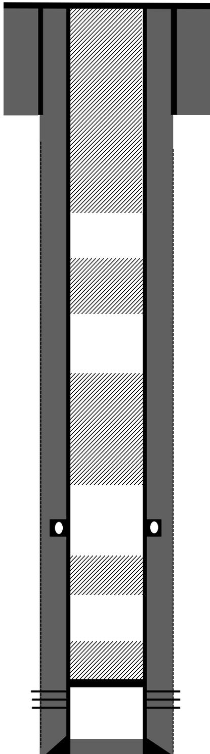
8-5/8" J-55 24# casing @ 238'. Cemented with 200 sks Class B. Circulated cement to surface. Hole size: 12-1/4
