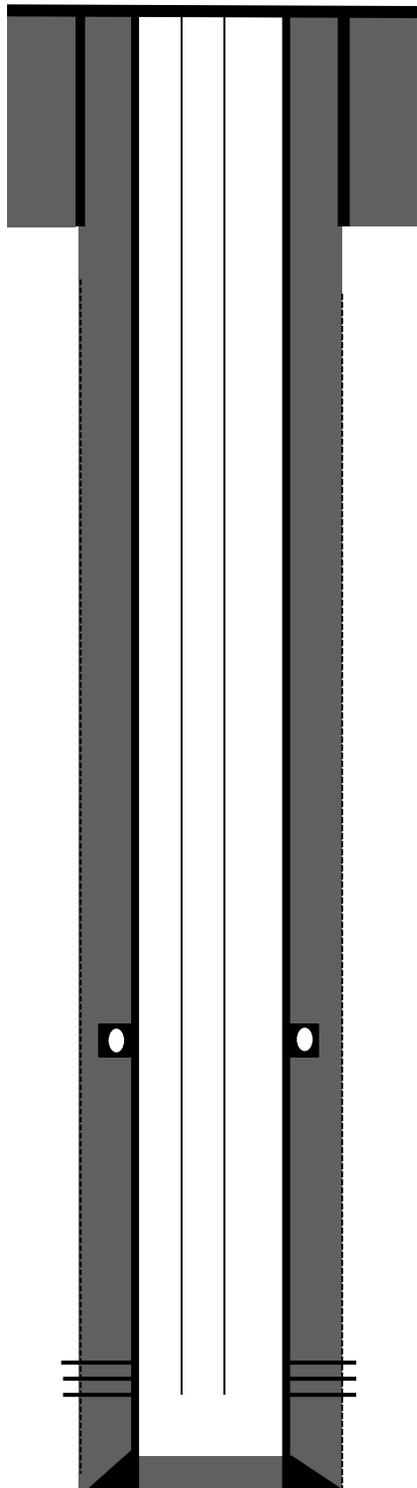
8-5/8" J-55 24# casing @ 238'. Cemented with 200 sks Class B.
