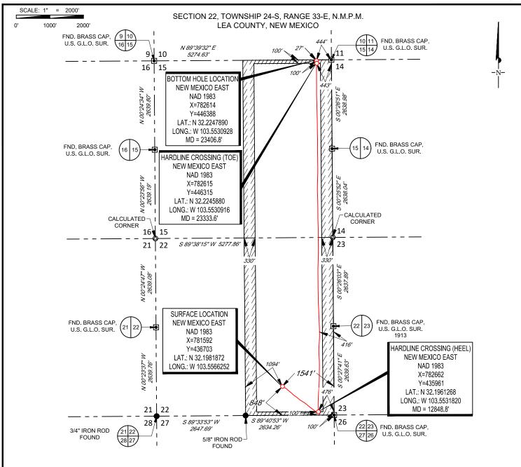
**JACKSON UNIT 928H** LEASE NAME & WELL NO .: \_ SECTION 22 TWP 24-S RGE 33-E SURVEY N.M.P.M. INTERNAL TION
