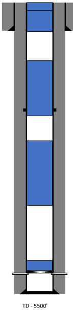
EOT @ 900'. PUMPED 70SX CL C CMT TO SURFACE. WOC. PUMPED 10SX TOP JOB. VERIFIED CMT TO SURFACE.
