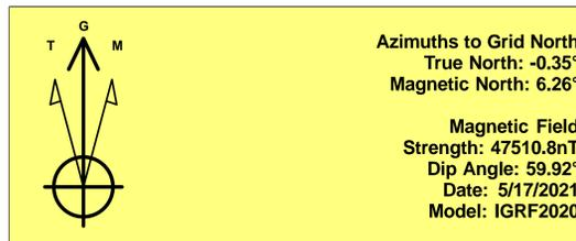
To convert a Magnetic Direction to a Grid Direction, Add 6.26°
