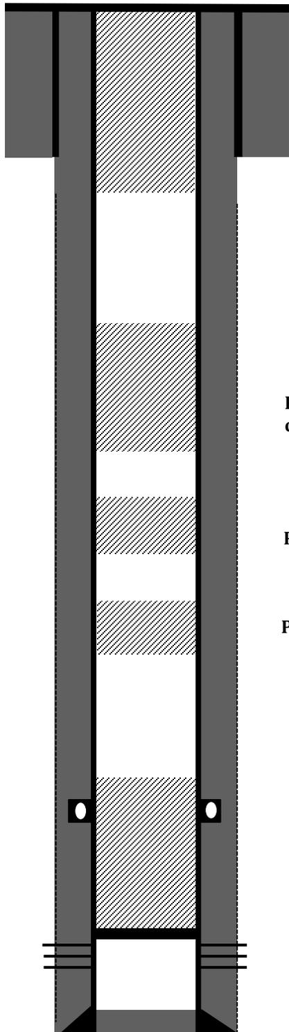
8-5/8" K-55 24# casing @ 213'. Cemented with 150 sks Class B.
