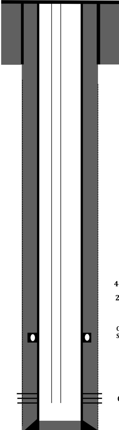
8-5/8" K-55 24# casing @ 213'. Cemented with 150 sks Class B.
