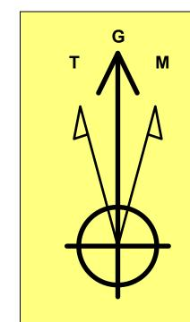
**Azimuths to Grid North** True North: -0.42° Magnetic North: 5.94°
