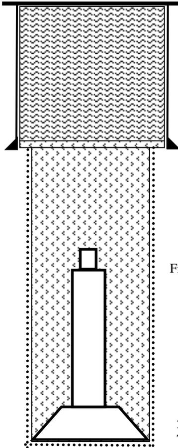
Filled cellar with  $\pm 29 \text{ yd}^3$  (785  $\text{ft}^3$ ) of dirt
